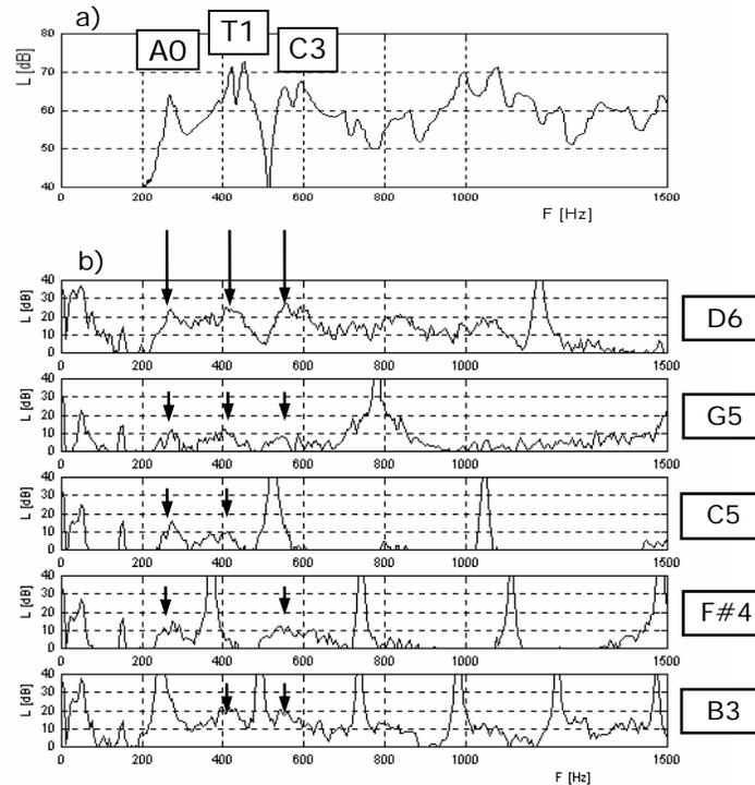
**Figure 5.** Comparison of the violin frequency characteristic (a) with time-averaged spectra of quasi-stationary part of tones (b) for the violin with high degree of *rustle*. Spectral signatures of violin modes A0, T1 and C3 in spectra are marked with arrows.
