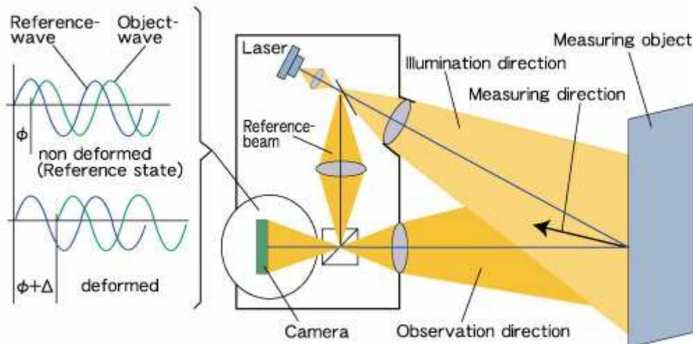
**Figure 2.** The basic principle of ESPI Q600
