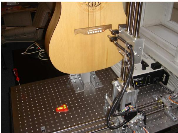
Figure 6. Automated carriage system
