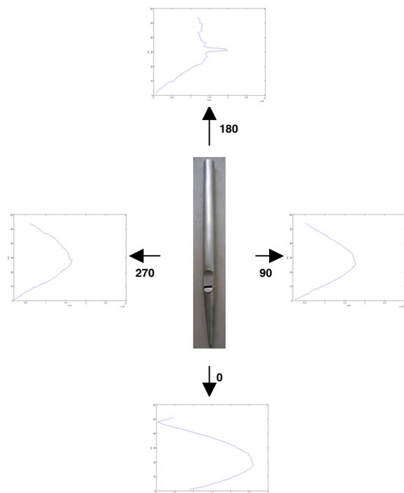
**Figure 3:** Wall vibrations of tin organ pipe for  $f = 256$  Hz
