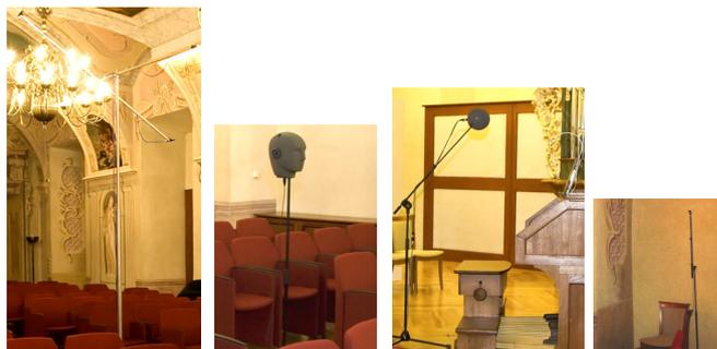
**Figure 1:** From left: 3 microphones above middle of usual listening places, dummy heads and microphone in an acoustic shadow.
