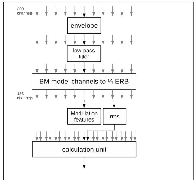
Figure 2. Block diagram of the central stage of the roughness model
