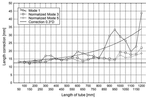
**Fig. 3** Dependencies of open-end length correction on the tube length with diameter 41.8 mm for three resonance modes
