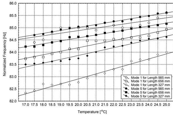
**Fig. 1** Dependencies of resonance modes 1 and 5 frequencies on air column temperature in three tubes
