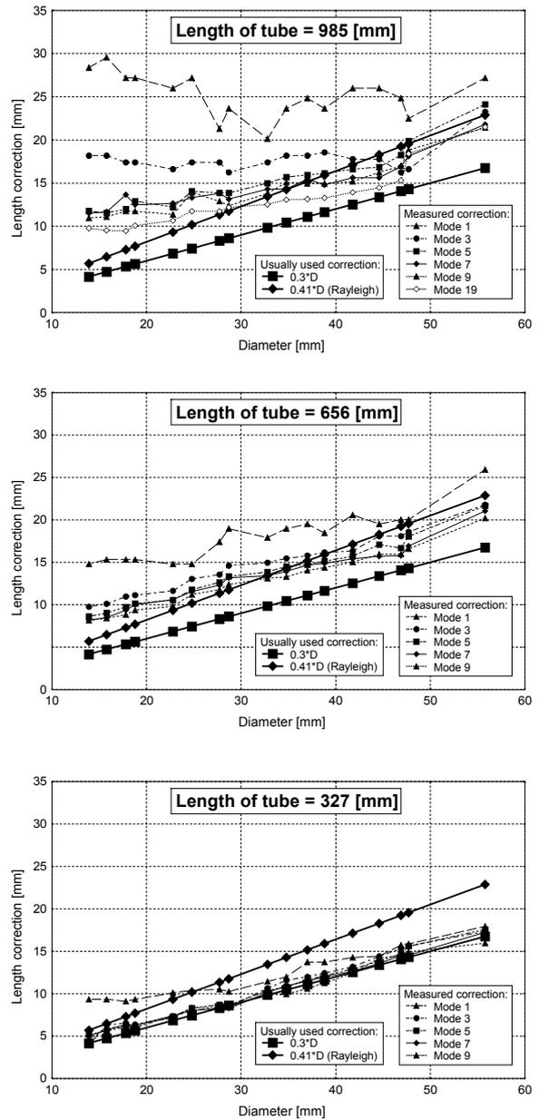
**Fig. 2** Dependencies of open end length correction on air column diameter for some resonance modes
