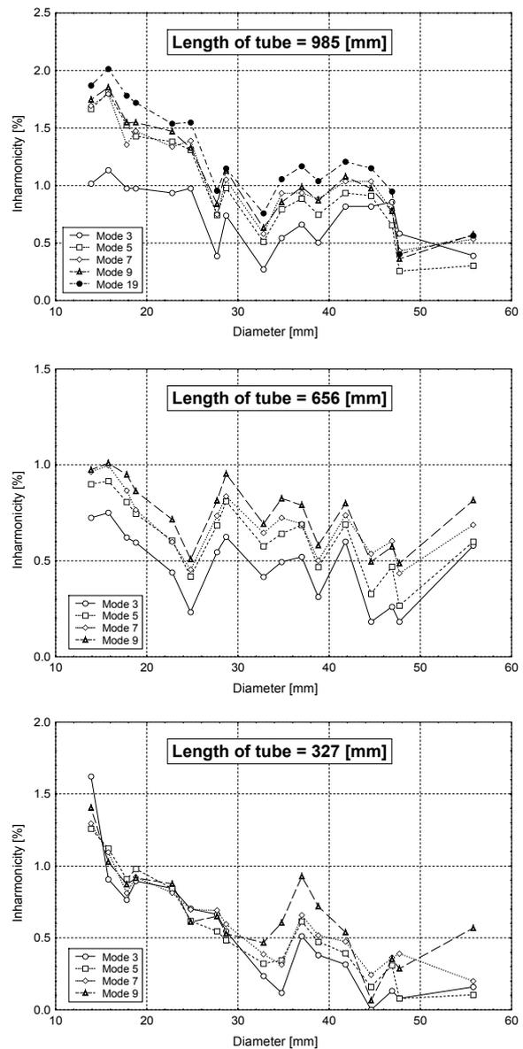
**Fig. 4** Dependencies of inharmonicity on air column diameter for some resonance modes
