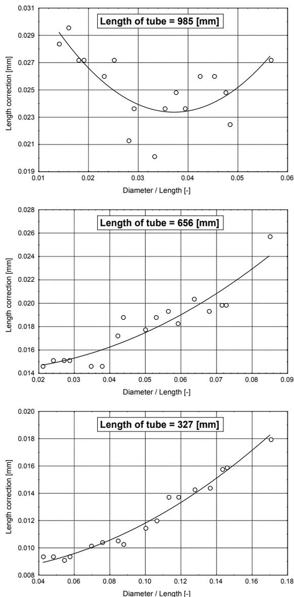
**Fig. 5** Dependencies of open-end length correction on the ratio of diameter to length for resonance mode 1
